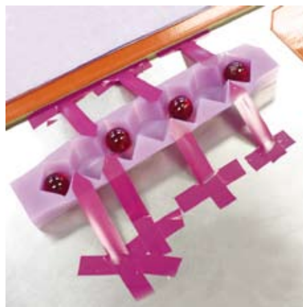
Great idea: Aaron Salvo used 3M™ Polyimide Film Electrical Tape to manipulate the shape of the 1" cube mold. Made of silicone, the tape's maximum operating temperature is 180° C or 356° F.
