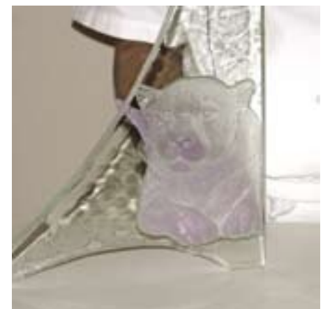
18. With care, the purple inclusion can be peeled from the casting.
